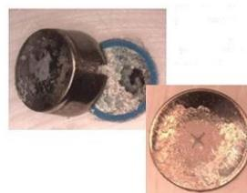
**Figure 1: Battery Leakage**
