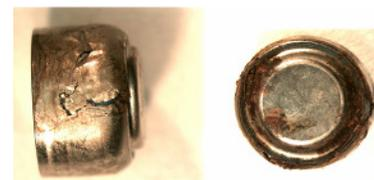
**Figure 2: Battery Corrosion**
